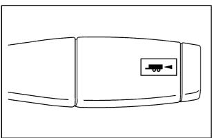
The vehicle has a Tow/Haul mode. The selector button is located on the end of the column shift lever. You can use this feature to assist when towing or hauling a heavy load or if there is a need to charge a battery installed in a trailer. See *Towing a Trailer on page 5-49* for more information.
